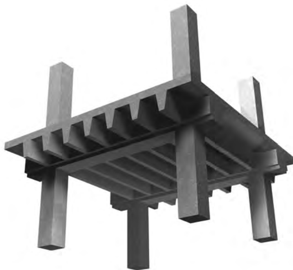
Figure 6.1 A wide-module joist system.
